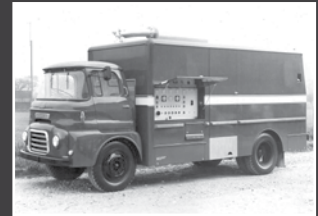
The 'L' range used in an Austin van, coupled to a Dale Electric set.
